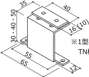
※1型枠 裏板16幅<br>TN枠 裏板10幅<br>FIX <N><br>
